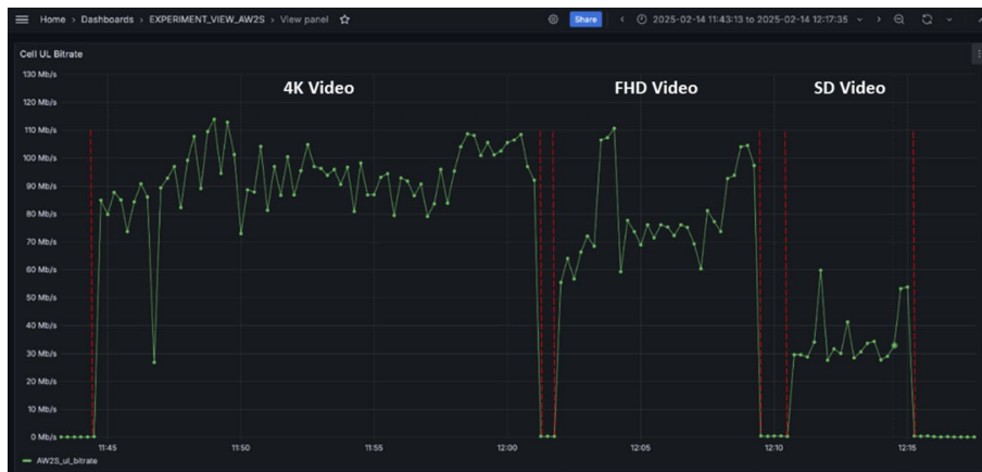
Fig. 5 Uplink bitrate variations during multiple resolution video streaming experiments
